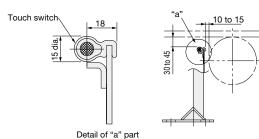
Dimension diagram of Transducer (mm)
