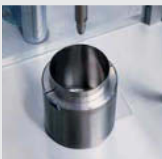
Stainless steel single-walled container located in the double-walled container receptacle
