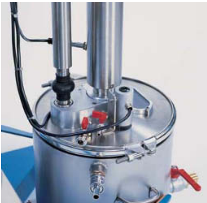
Vacuum cover with vacuum and exhaust connections, halogen light, scraper with cardan and gear unit
