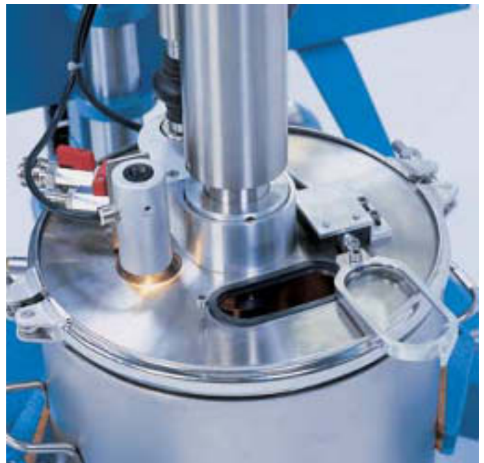
The generously sized slewing inspection glass simultaneously serves as an opening for product feed; when the inspection glass is opened, the scraper system automatically shuts off.
