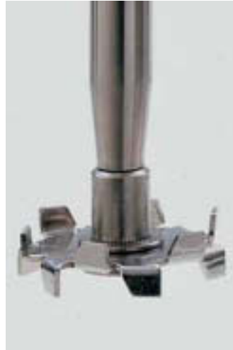
Heavy duty stainless steel dispersion impellers, with tooth profile, with 5mm hole, sizes available: 30, 40, 50, 60 mm Ø; Hub and female thread, sizes available: 70, 80, 90, 100, 125 and 150 mm Ø; with adapter, sizes available 175 und 200 mm Ø.
