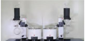
Main unit + Glassware set B The device is operated by the control panel located in the center. Turning the encoder (knob) slowly adjusts the number of revolutions display by one rpm, and turning it fast by ten rpm. The rotational speed can be set within the wide range of 5 to 315 rpm. After confirming the rpm value, press the ► ■ keys to rotate the distillation flask. The rotation mode can be selected from forwards rotation, reverse rotation,
